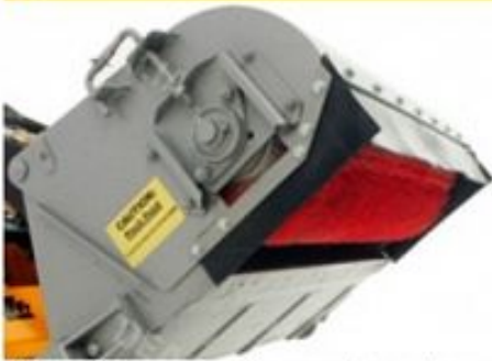
Hi performance forward and reverse bucket broom.
